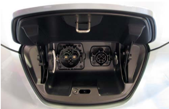
Figure 5. The standard J1772 receptacle (right) can receive charge from Level 1 or Level 2 equipment. The CHAdeMO DC fast charge receptacle (left) uses a different type of connector. Photo by Andrew Hudgins, NREL/PIX 19558
